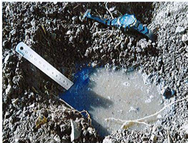
Figure 2: Step 2 of percolation test
