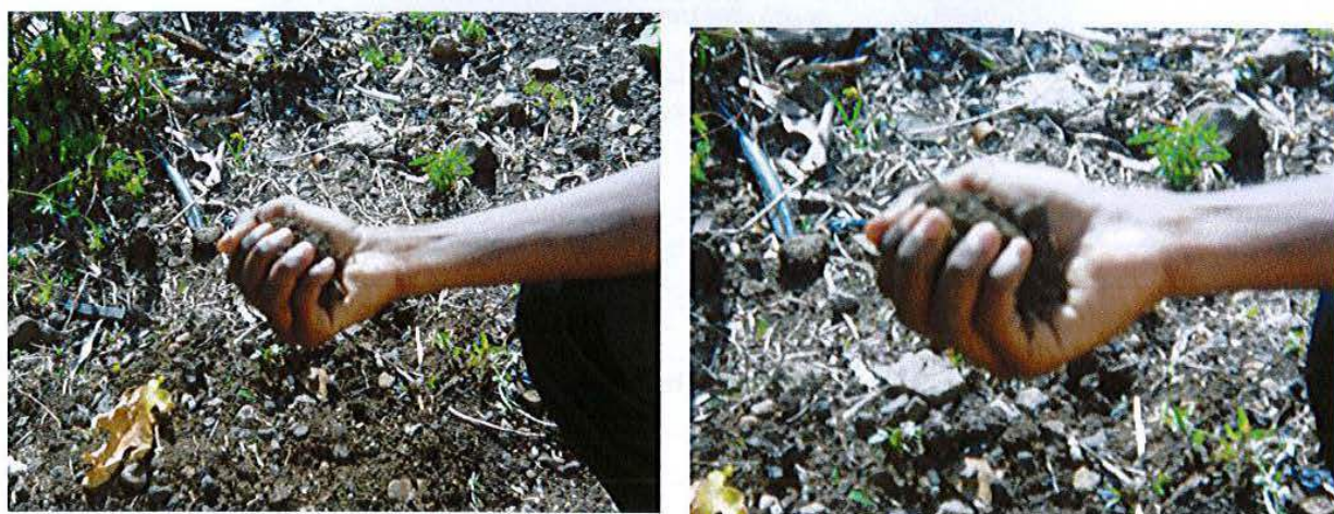
Fig 2.2: Step 2 of squeeze test
